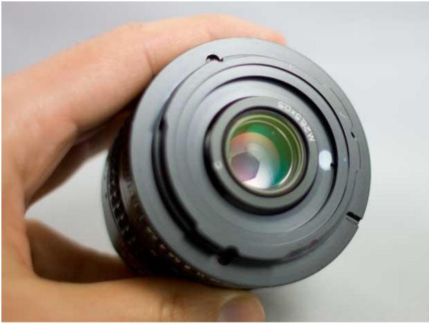
Picture the size of the fins, visible here inside this lens, when trying to understand the concept of f-stops.
